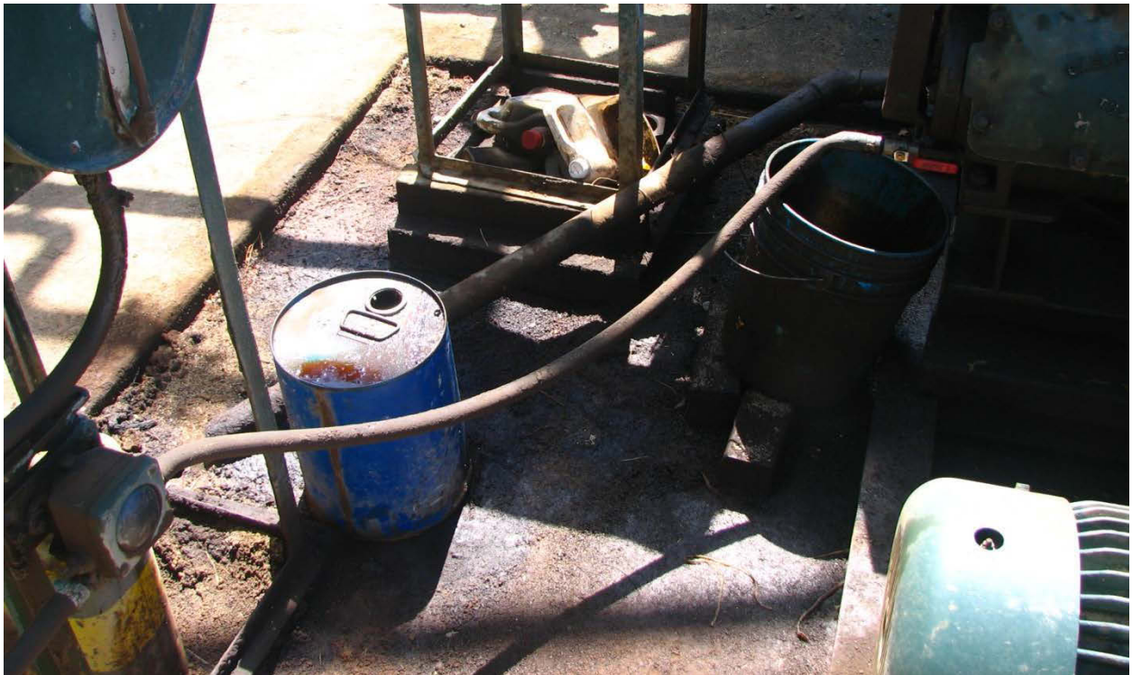
Several open containers of hazardous fluid were observed near the tank battery.
